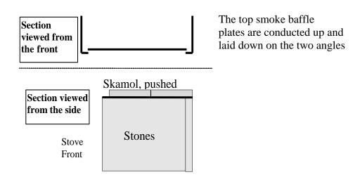
The bottom smoke baffle plates (Skamol) are pushed in over the stone holders and in to the rear wall.
