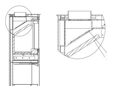
Steel smoke baffle plate Skamol smoke baffle plate
