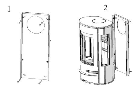
The stove is hung on the wall bracket. (2-3) The locking screw is tightened. (4)
